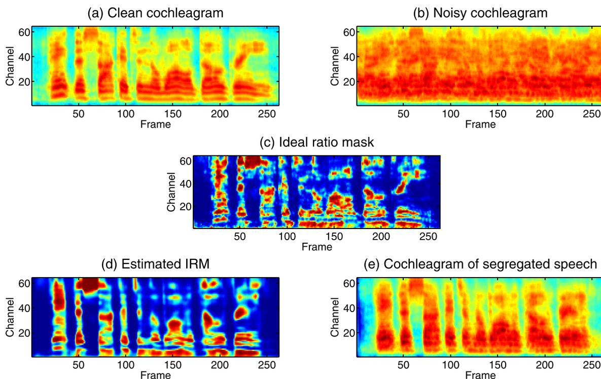
FIG. 2. (Color online) Segregation of an IEEE sentence (“Paint the sockets in the wall dull green”) from babble noise at  $-5$  dB SNR; (a) the cochleagram of the utterance in quiet; (b) the cochleagram of the speech-plus-noise mixture; (c) the IRM for this mixture; (d) the IRM for this mixture estimated by the algorithm; and (e) the cochleagram of the utterance after applying the estimated IRM to segregate the speech from noise.
